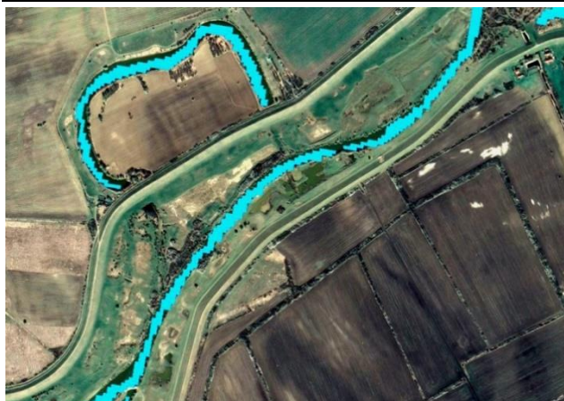
Fig. 4: Small ditches south of Bârzava River (light blue pixels) which could not be mapped because of their width smaller than a Sentinel-2 pixel
