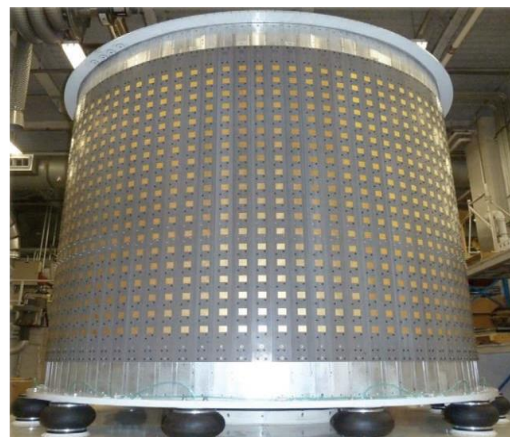
Fig. 7: Cylindrical Polarized Phased Array Radar (Mark, 2014)
