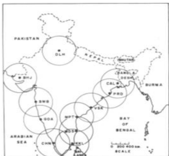
Fig. 3: The network of radars in the S-band of India Meteorological Department (Atlas, 1990)
