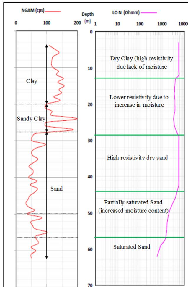
Fig. 6: Interpreted gamma ray and resistivity logs showing a sequence of clay, sandy clay and sand
