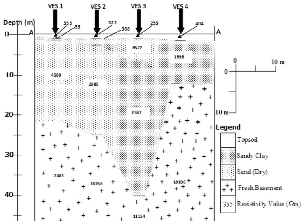
Fig. 5a: Geoelectric sections along profile A - A'
