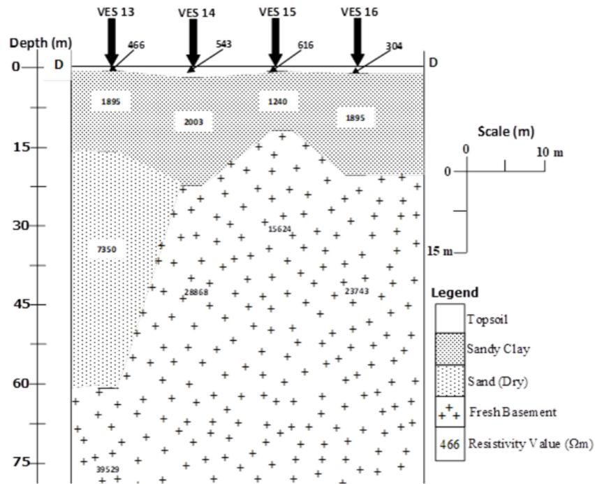
Fig. 5d: Goelectric sections along profile D - D'
