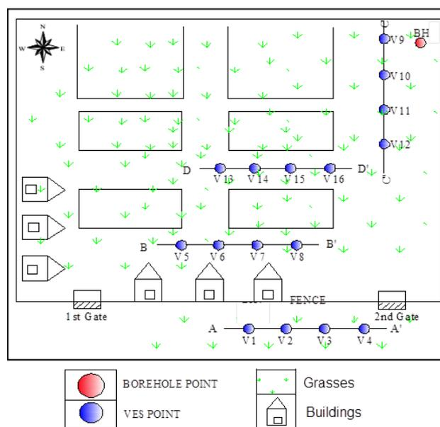
**Fig. 2: Location of Vertical Electrical Soundings and geologic logging test**
