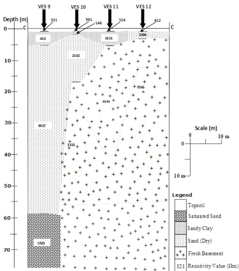
Fig. 5c Geoelectric sections along profile C - C'
