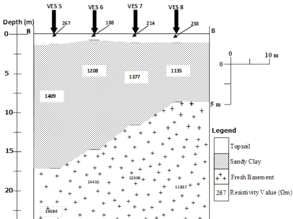
Fig. 5b: Geoelectric sections along profile B - B'
