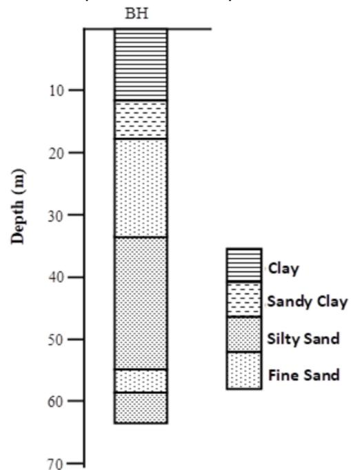
**Fig. 3: Stratigraphic log of drill at the north-eastern part of the study area**
